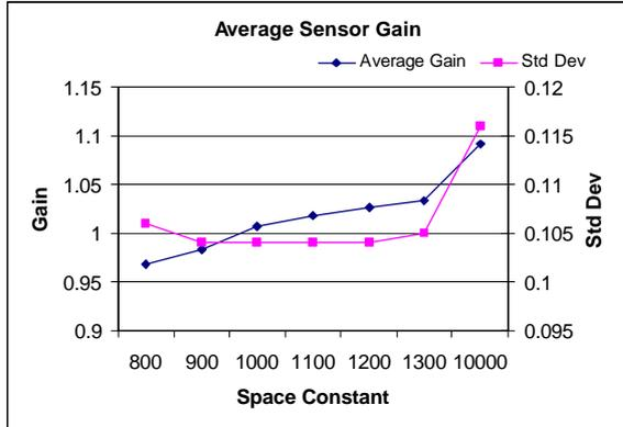
**Figure 2** Average sensor gain and standard deviation for various propagation model parameter values
