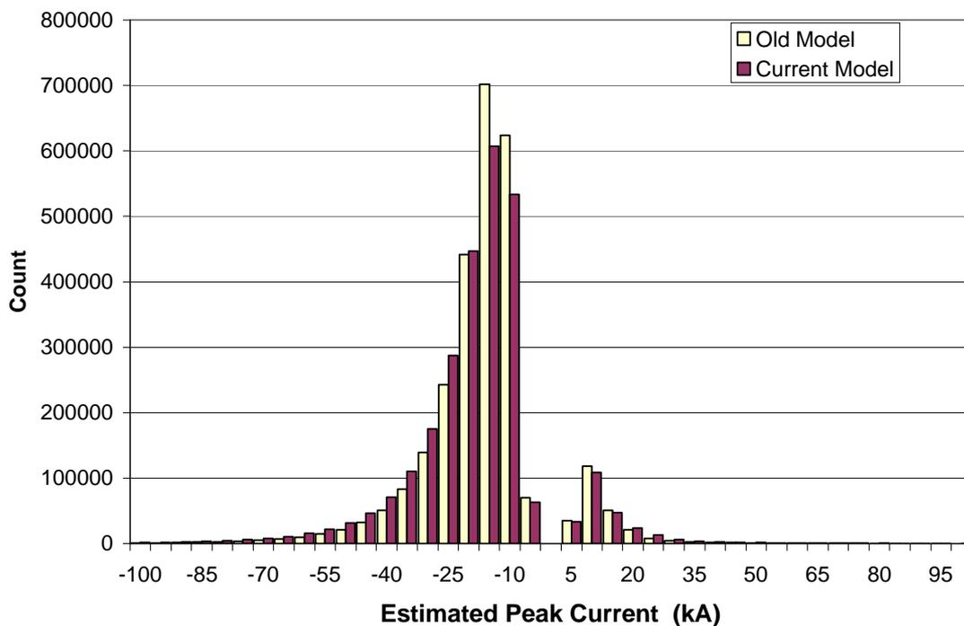
**Figure 4** Sample estimated peak current distribution from the central US illustrating the effect of changing the propagation model parameters.
