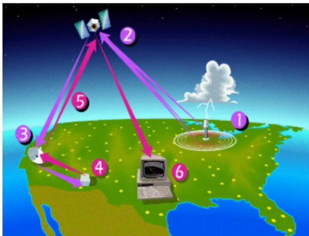
**Figure 1** Communications data flow in the NLDN. Actual system employs three satellite down-link locations represented by item (3).
