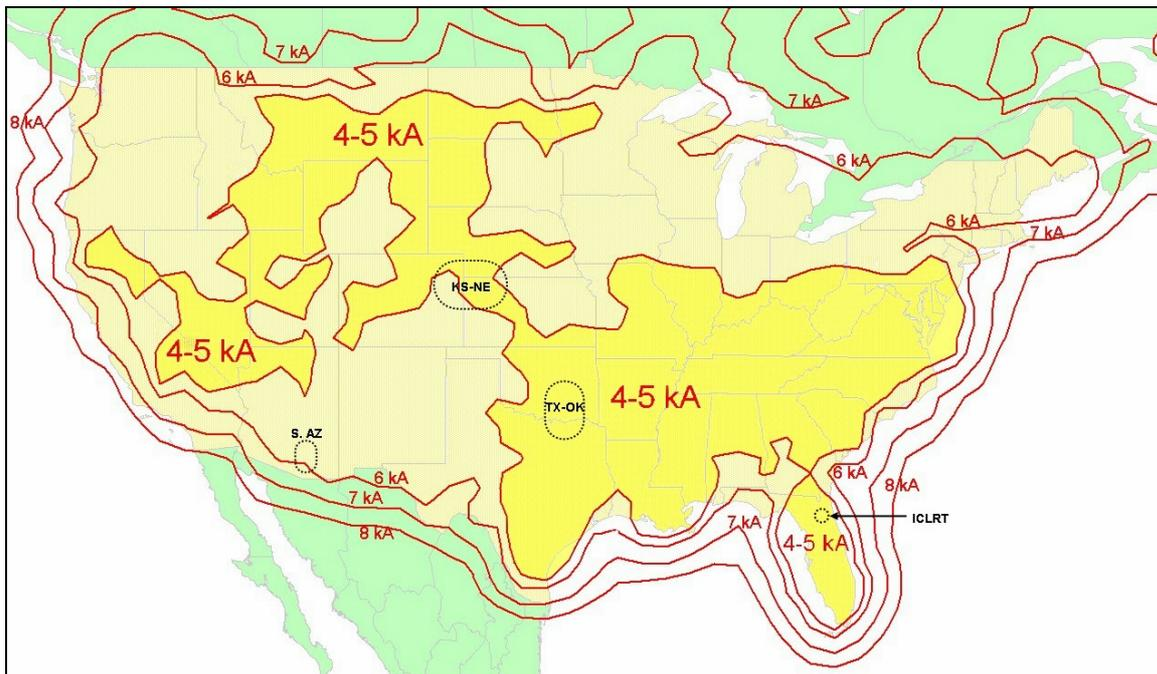
**Figure 5** Estimated minimum detectable peak current for the upgraded NLDN. Validation studies in 2003-4 were carried out in the four small regions identified by black circles.
