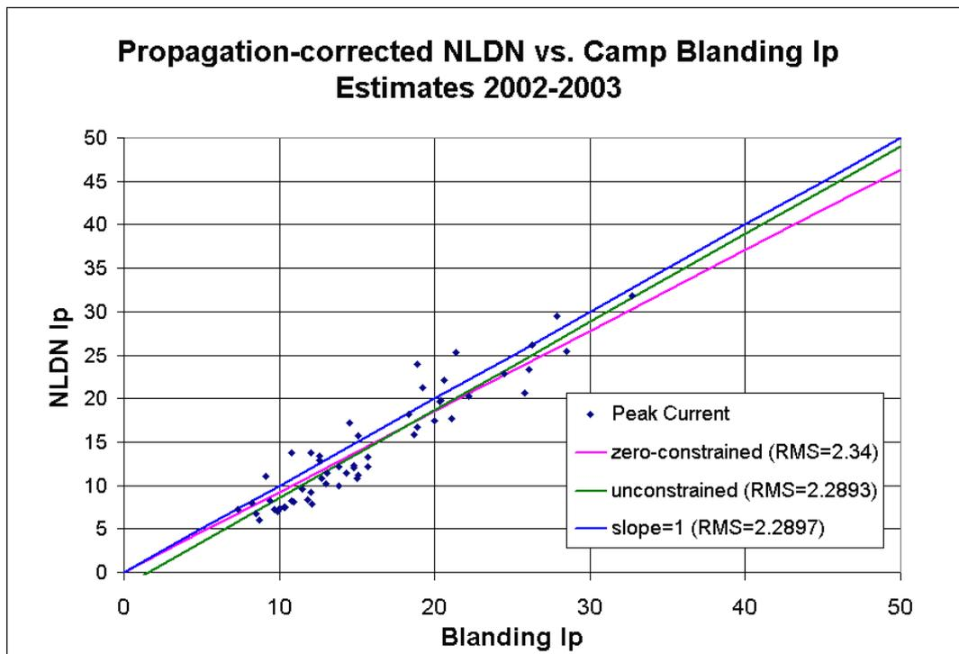
**Figure 3** Scattergram of NLDN estimated peak current (kA) vs measured rocket-triggered lightning peak current for 55 subsequent strokes from 2002-2003. Various regression lines and related RMS deviations are shown (see inset for details)
