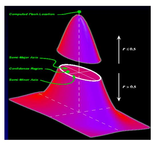
When measurement errors are purely random, the error in the location is described by a 2-D Gaussian with the optimized position at the peak. The location accuracy is defined as the semimajor axis of the elliptical region formed by cutting the probability distribution at the 50% level.
