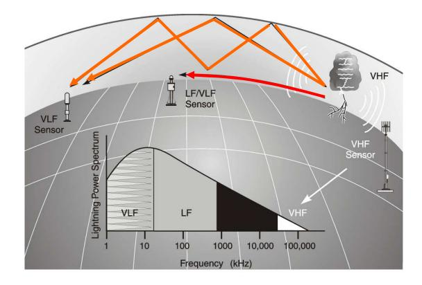
NLDN sensors are broadband: The "normal" CG lightning data set is produced by detecting ground wave signals (red path). In addition, the sensors also respond to ionosphericallypropagated electromagnetic signals coming from long distances (orange path) that have the LF components filtered out by the propagation.
