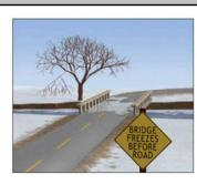
The bridge would become icy first because it would lose heat energy over its entire surface. The bridge would cool by radiative heat transfer to the air from its top, its sides and its underside. The net effect is that the bridge's temperature would closely mirror the air's temperature at night.
