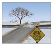
The bridge would become icy first because it would lose heat energy over its entire surface. The bridge would cool by radiative heat transfer to the air from its top, its sides and its underside. The net effect is that the bridge's temperature would closely mirror the air's temperature at night.
