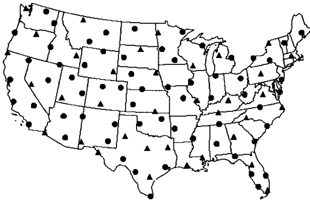
Fig. 2. The locations of lightning sensors in the NLDN: triangles show IMPACT sensors and the circles show LPATS sensors. (Adapted from [47].)
