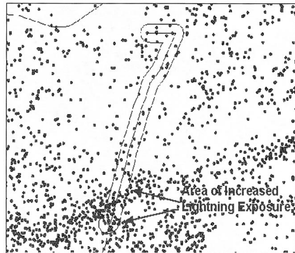
Fig. 10. A map of the CG strokes that struck in the region of a 32-mile 115-kV transmission line in 1995 in Minnesota. Note that in this year, there were two areas that had high exposure to lightning. The flashes plotted in bold were located within 2.5 km of the line. (Adapted from [74] and [75].)
